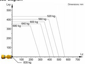
The KR 640 R2800-2 is designed for a rated payload of 640 kg in order to optimize the dynamic performance of the robot. With reduced load center distances and favorable supplementary loads, a maximum payload of up to 835 kg can be mounted. The specific KUKA Load case must be verified using KUKA. For further consultation, please contact KUKA Service.
