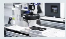
**Gluing.** In bonding and 3D bonding applications, various requirements come together: Different gripping positions must be localized, paths must be followed accurately and target positions must be addressed precisely. Automating adhesive bonding processes greatly reduces the error rate.
