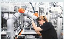
**Fasten.** Especially in ergonomically unfavorable locations, such as inside electrical appliances, robots play an important role in screw fastening in terms of ensuring employee health and fast cycle times. Material tolerances are compensated with the aid of a vision system.
