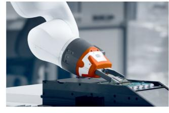
**ESD robots.** ESD robots ideally protect against electrostatic charging or discharging. From assembly to inspection and packaging of electronic consumer goods – KUKA offers various robot series in ESD design with electrically conductive elements and surfaces as standard for electronics production.
