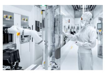
CR robots. KUKA offers three robot types for use in cleanrooms: the KR AGILUS CR, the KR CYBERTECH CR and the LBR iiwa CR. Airborne particles are avoided and, thanks to special seals, the robot does not generate dust or particles caused by seal abrasion.
